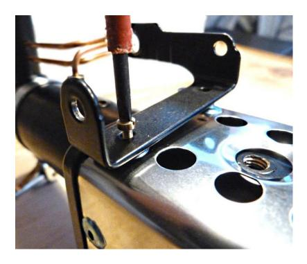
Screw down onto the two pre-fitted nuts.
