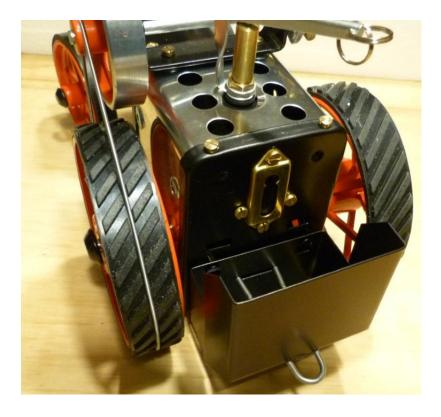
Screw the Safety Valve into the boiler top. This is the hole for the water.
