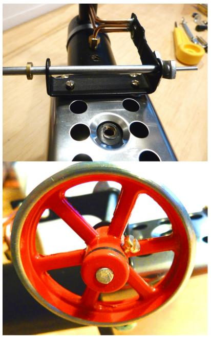
Don't forget the brass spacer, and then fit the Flywheel and tighten the brass securing screw.
