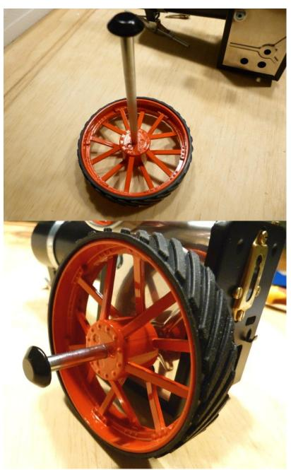
Fit the black Hub Cap onto one end of the rear axle, insert through the Cowl axle hole and then fit the other wheel and Hub Cap (bit of a hard push).
