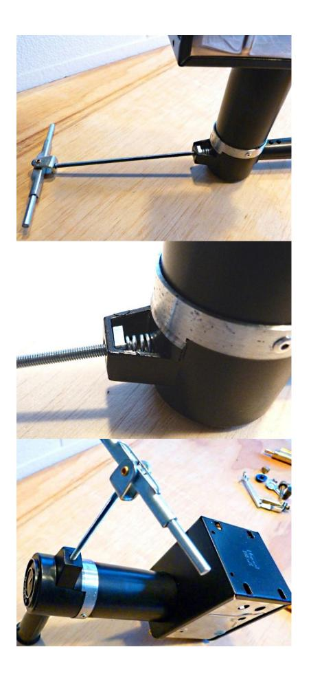
Screw the Forks assembly until it is in contact with the Smoke Box base.
