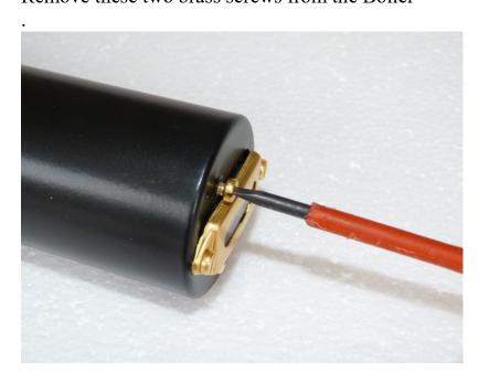
Then feed the Boiler into the Firebox assembly so that its Water Level brass surround fits neatly into the shaped hole on the other face. Now use the two brass screws to secure it to the Firebox. Don't scratch it by allowing your screwdriver to slip – be gentle.
