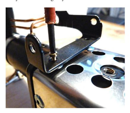
Screw down onto the two pre-fitted nuts.
