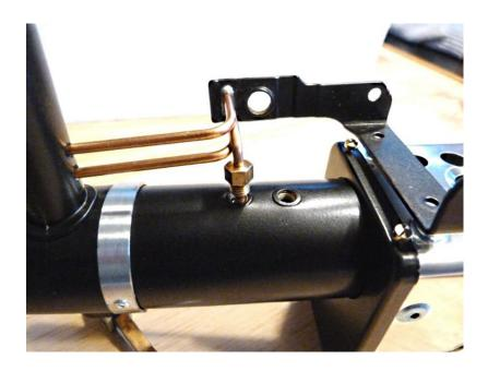
You may have to "persuade" this Engine Face Mounting Bracket to get the two pipes, the boiler pipe and the two holes all lined up. Use your muscles – gently.
